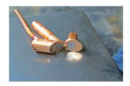
**ASIWELD** exothermic welding is a simple, efficient, high quality metal connection method exothermic welding by alumino-thermic reaction generated by high temperature to make metal molten completely, to achieve high quality welding effect. This reaction is conducted in the graphite mould of high temperature resistance; normally a graphite mould could be used for more than 80 points. Exothermic reaction process takes a few seconds only.
